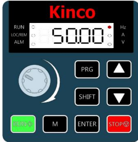
Figure 4-6 AC drive power-on display
