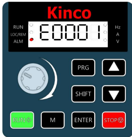
Figure 6-1 The interface fault display
